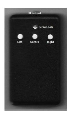
The TL-Lite is a Intervalometer or time lapse timer for Olympus range of IR enabled cameras. The TL-Lite measures (65x35x24mm) weighs 30 grams and is powered by one 3 volt CR2032 battery. Battery life over 300 hour's continuous use with the unit set at one shutter trigger every 4 seconds.
