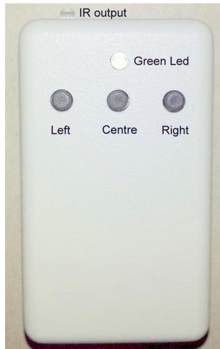
The TL-Lite is a Intervalometer or time lapse timer for Nikon's DSLR range of IR enabled cameras. The TL-Lite measures (65x35x24mm) weighs 30 grams and is powered by one 3 volt CR2032 battery. Battery life over 300 hour's continuous use with the unit set at one shutter trigger every 4 seconds.
